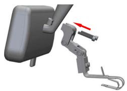
**5 - Install the mount while sitting in the passenger side of your vehicle.** Remove the two socket head screws so the top portion of the mount may be removed. Position the mount on the bottom of the stem as shown above. Reattach the top portion of the mount. Tighten both screws evenly making sure it is in the correct position as shown above. Tighten both screws until mount is securely attached to the mirror stem.
