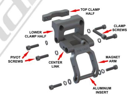
4 - Remove the two socket head CLAMP SCREWS as shown above. Loosen the hinge PIVOT SCREWS to position mount as desired. Remove the ALUMINUM INSERT and screws to instal the magnet onto the MAGNET ARM.
