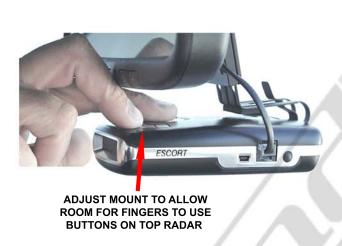
7 - Install the RD onto the mount. Make the necessary adjustments as shown above. Using the upper and lower pivots, and the vertical adjustment, leave enough room below bottom of mirror to allow access to buttons on top of radar detector.
