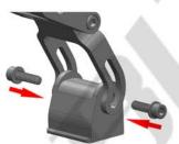
3 - Install aluminum threaded insert into magnet, and attach magnet onto blendmount with lip pointed in direction as shown.
