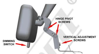
6 - Install the RD onto the mount. We recommend you adjust the RD so it is as close to the bottom of the mirror as possible. Using the vertical adjustment and orienting the double pivot center link, adjust RD upward as far as possible while making sure the mirror dimming switch is still accessible. After all adjustments are made, be sure to check that the pivot and vertical adjustment screws are tight. Grab the long arm of the allen wrench to assure that these screws are securely tightened.
